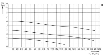
PA = Output pressure PE = Input pressure Q = Flowing through I Inlet pressure sensivity
